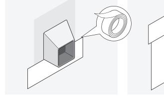
Apply flashing to the bottom of the<br/>penetration. We recommend usingApply flashing along the sides and then<br/>the top, shingling each layer.Barricade Flash Ulti, Barricade FlashHe top, shingling each layer.
