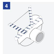
Tape over the 45° cuts using Barricade Seam Tape.
