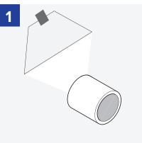
Cut two 45° angles and peel back house wrap above the penetration.
