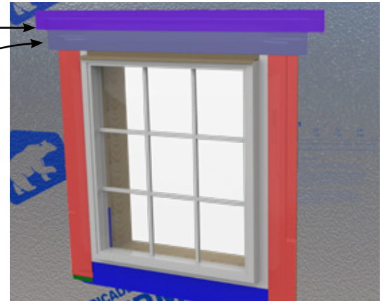
Step 8: Install trim boards and fasten to the furring strips or substrate.
