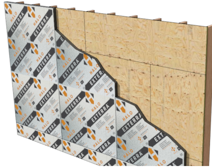
Offset horizontal and vertical joints between Exterra and wood sheathing when possible.
