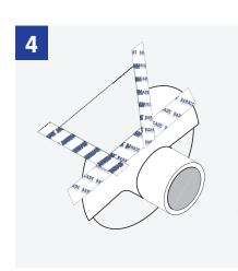
Tape over the  $45^\circ$  cuts using Barricade Seam Tape.
