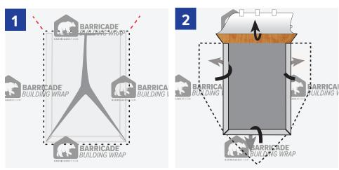
Make an inverted Y-cut in the wrap at window rough opening. Make diagonal cuts at the top of the rough opening corners. Windows must be installed according to the manufacturer's recommended installation process. Fold the three flaps in through the opening, fastening them inside with staples set about every 6". Fold top flap up and tape temporarily as shown. Proceed to flashing installation (page 8).
