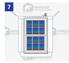
A. Release the tape and drape the upper WRB flap onto the window header.B. Trim across the flap to allow at least 1" overlap of the header flashing.
