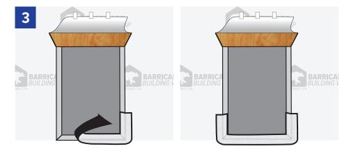
Prepare sill flashing by cutting Barricade Flash Conform at least 12" longer than the width of the rough opening. Install sill flashing by removing the release paper, centering sill flashing on sill framing stud, and adhering into rough opening. The back edge of Flash Conform should extend to inside edge of sill framing stud and at least 6" up each jamb framing stud. (Sill flashing should not wrap onto the inside of wall.)
