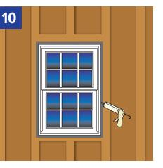
Complete the window installation following manufacturer's instructions. Apply a bead of sealant all the way around the window frame and the window opening. If the gap is larger than 3/8" the use of a foam backer or a low expansion foam is acceptable. Do not use a high expansion foam as it can warp the window frame. When using sealants or primers, be sure Barricade branded (or compatible) sealant is used.
