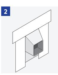
Apply Barricade Window flashing along the sides first, leaving the bottom unflashed. Next apply Barricade Window flashing over the top, shingling the side flashing.
