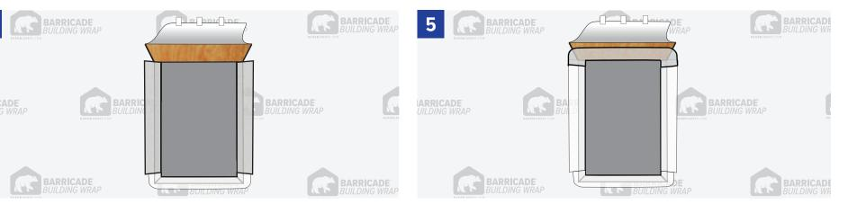
A. Cut Barricade flashing material to fit within the vertical length of the rough opening.B. Remove the backing and apply the vertical flashing to cover the wood framing and fold onto the exterior face of the wall adhering to the WRB.
