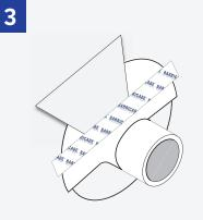
Replace building wrap flap over the flashing and tape across using Barricade Seam Tape.
