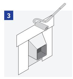
Use a roller to apply even pressure along the flashing, being sure to push out any air pockets that may have appeared. Barricade suggests finishing with Barricade Construction Sealant to ensure a tight seal around the edges of the penetration.
