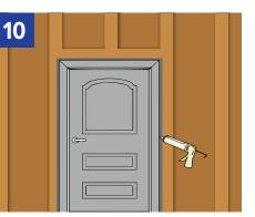
Complete the door installation following manufacturer's instructions. Apply a bead of sealant all the way around the doorframe and the window opening. If the gap is larger than 3/8" the use of a foam backer or a low expansion foam is acceptable. Do not use a high expansion foam as it can warp the door frame. When using sealants or primers, be sure Barricade branded (or compatible) sealant is used.
