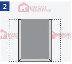
**A.** Flip the cut head flap upward to expose the sheathing and temporarily secure with Barricade Seam tape.
