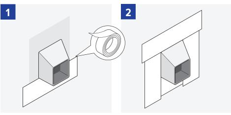
Apply Barricade Window flashing to the bottom of the penetration.
