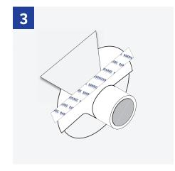
Replace building wrap flap over the flashing and tape across using Barricade Seam Tape.
