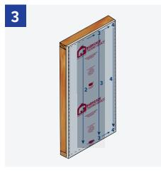
Moving across the panel, attach fasteners at the top and bottom of the panel until you reach the next stud. (Note: when using staples, it's important to fasten them in a parallel direction to the stud.)
