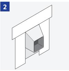
Next apply Barricade Window flashing over the top, shingling the side flashing.
