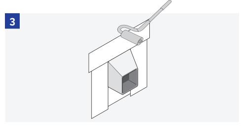
Use a roller to apply even pressure along the flashing, being sure to push out any air pockets that may have appeared. Barricade suggests finishing with Barricade Construction Sealant to ensure a tight seal around the edges of the penetration.
