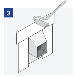
Use a roller to apply even pressure along the flashing, being sure to push out any air pockets that may have appeared.
