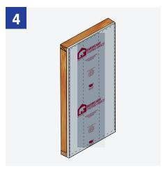
Fasten panel in numerical order repeating the procedure described in steps 2 and 3. Continue until the Thermo-Brace panel is properly secured to the frame.
