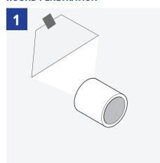
Cut two 45° angles and peel back building wrap above the penetration.
