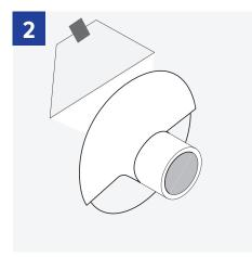
Apply Barricade Flash Conform to the underside of penetration, shingling the above side after. Use a roller to apply even pressure along the flashing.
