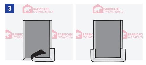
Prepare sill flashing by cutting Barricade Flash Conform at least 12" longer than the width of the rough opening. Install sill flashing by removing the release paper, centering sill flashing on sill framing stud, and adhering into rough opening. The back edge of Flash Conform should extend to inside edge of sill framing stud and at least 6" up each jamb framing stud. (Sill flashing should not wrap onto the inside of wall.)
