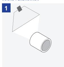
Cut two 45° angles and peel back building wrap above the penetration.
