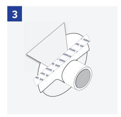
Replace building wrap flap over the flashing and tape across using Barricade Seam Tape.
