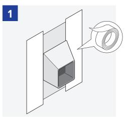
Apply Barricade Window flashing along the sides first, leaving the bottom unflashed.
