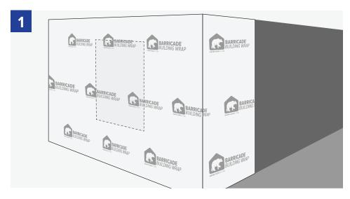
Start by placing the roll 2-3 feet from the corner and fasten using plastic cap nails or staples (best practice), staples, large-headed nails or roofing nails spaced a maximum of 18 inches on center.
