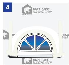
Follow above instructions for proper installation pro to head flashing installation. Install circular-top windows according to window manufacturers installation guidelines, then follow instructions below to complete the process.
