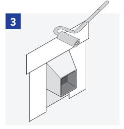
Use a roller to apply even pressure along the flashing, being sure to push out any air pockets that may have appeared.
