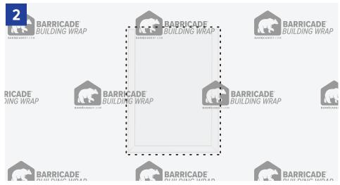
Unroll the wrap around the building and fasten with plastic cap nails or staples (best practice), staples, large-headed nails or roofing nails spaced a maximum of 32 inches on center.
