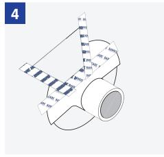
Tape over the 45° cuts using Barricade Seam Tape.
