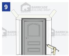
Apply sealant along the top and sides of the door between flashing tape and window frame. Do not apply sealant along the bottom of the window to allow water a place to drain.
