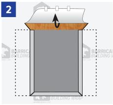
**A.** Flip the cut head flap upward to expose the sheathing and temporarily secure with Barricade Seam tape.
