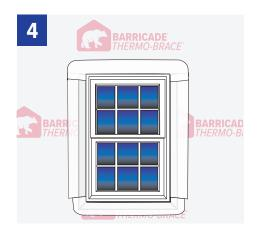
Install and shim window into rough opening per manufacturer's instructions. When using sealants or primers, be sure Barricade branded (or compatible) sealant is used.
