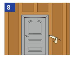
Complete the door installation following manufacturer's instructions. Apply a bead of sealant all the way around the doorframe and the window opening. If the gap is larger than 3/8" the use of a foam backer or a low expansion foam is acceptable. Do not use a high expansion foam as it can warp the door frame. When using sealants or primers, be sure Barricade branded (or compatible) sealant is used.
