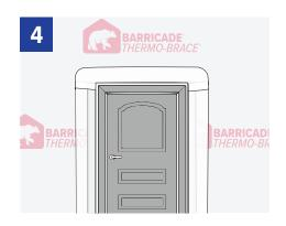
Install and shim door into rough opening per manufacturer's instructions. When using sealants or primers, be sure Barricade branded (or compatible) sealant is used.
