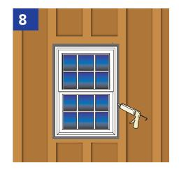
Complete the window installation following manufacturer's instructions. Apply a bead of sealant all the way around the window frame and the window opening. If the gap is larger than 3/8" the use of a foam backer or a low expansion foam is acceptable. Do not use a high expansion foam as it can warp the window frame. When using sealants or primers, be sure Barricade branded (or compatible) sealant is used.
